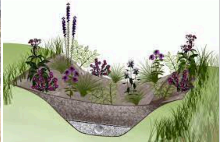
Vegetated Bioswales Filter, slow down, recharge stormwater
